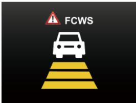
P.S. LDWS and FCWS features need to have GPS fixed first, and under enough light environment to activate the system. Under night time or low light environment, it will affect the detection, and while raining it will also affect the detection.
